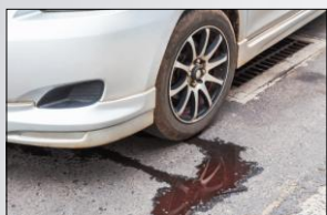
Oil and other fluids leaked or spilled on paved areas carried by storm water into the storm drain system.
